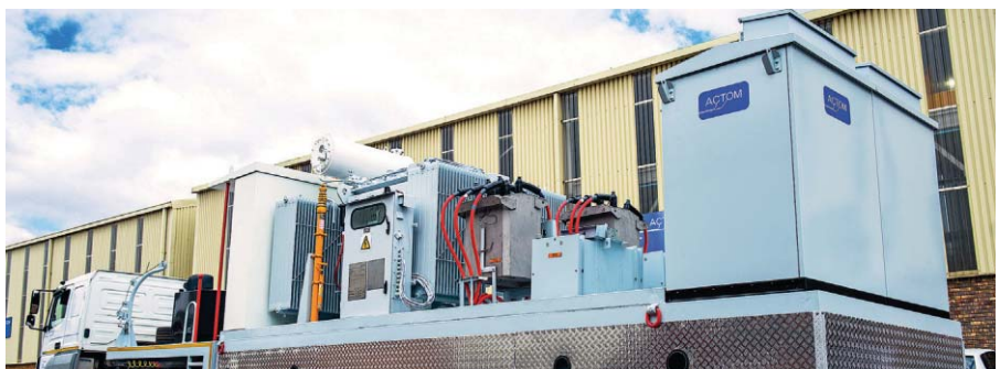
ACTOM Mobile Substation
