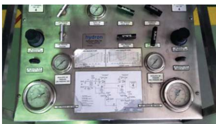
High pressure water testing equipment
